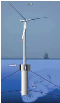
Oxygenation pumping in open sea powered by windmills (conceptual stage).
