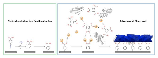
The synthetic strategy to produce HKUST-1/graphene conductive coatings on top of glassy carbon electrodes (drawn as grey rectangles) is displayed. For simplicity, charges are not shown, and the structural components are not on scale.
