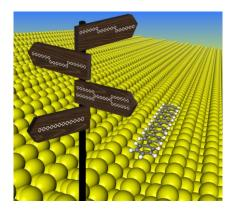
**Fig. 1** Controllable fabrication of linear polyphenyl wires by direct C–H activation and C–C coupling of para-sexiphenyl (p-6P) has been achieved on an anisotropic Au(110) surface. Owing to the one-dimensional spatial constraint at the surface, the equivalent C–H bonds of p-6P molecules are differentiated with various reaction probabilities.
