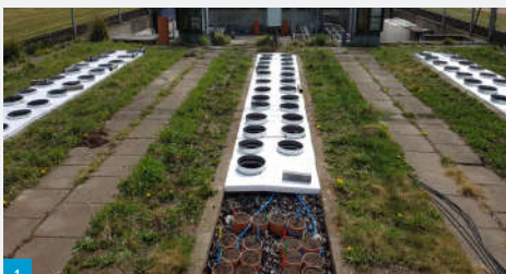
1) Experimental mesocosm set-up (semi-field) to determine spatial differences of GHG flux dynamics of five Danish peatlands.
