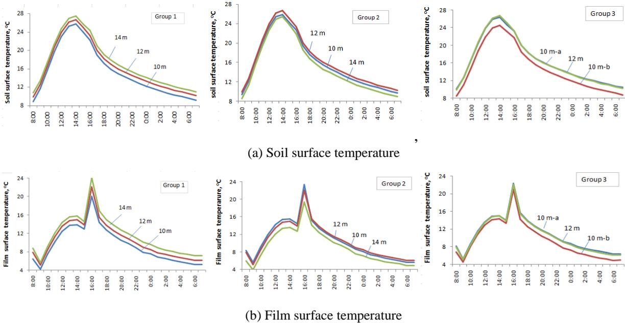
Figure 6. CSG indoor soil and film surface temperatures
