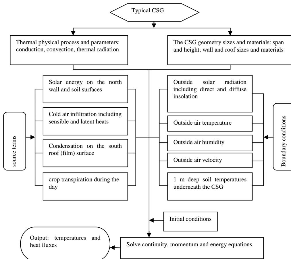
Figure 4. CSG simulation procedure and models
