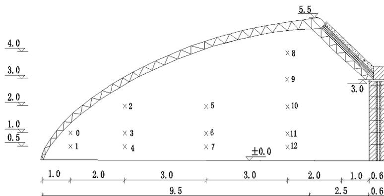
Figure 2. Air temperature measurement points with dimensions in meters
