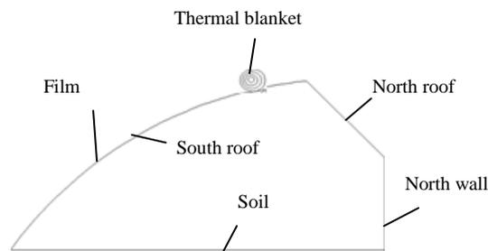
Figure 1. CSG picture and names of the components
