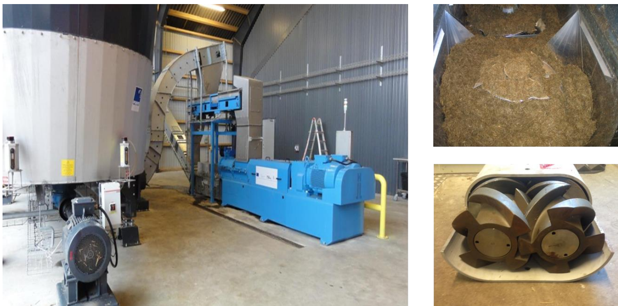
Figure 1. The extruder and the mixer for feeding in of biomass. At the right, a look into the mixer and a close up photo of the two co rotating screws.
