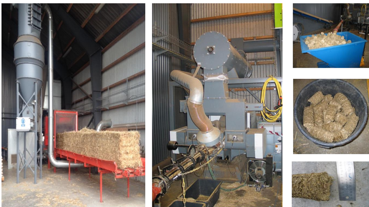
Figure 2. The shredding and briquetting set up. At the right, the produced briquettes.
