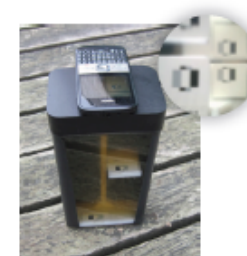
Secchi3000 and a mobile phone on the top of the device. Inside the container there is the measurement structure with plates consisting of white, grey and black target areas.
