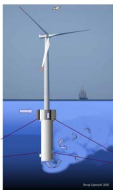
Oxygenation pumping in open sea powered by windmills (conceptual stage)
