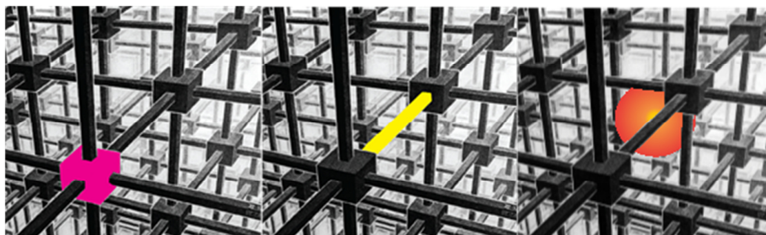
Figure 1 From left to right: Modification of the cationic unit; of the linker and embedding of a guest material in the pores.
