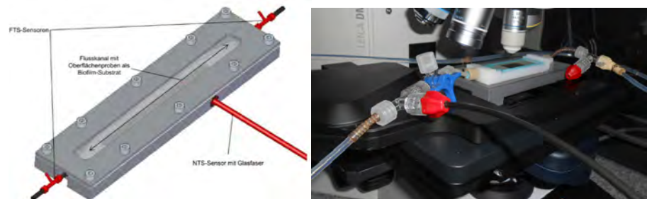
Fig. 1: Set-up for online biofilm monitoring in a CLSM system
