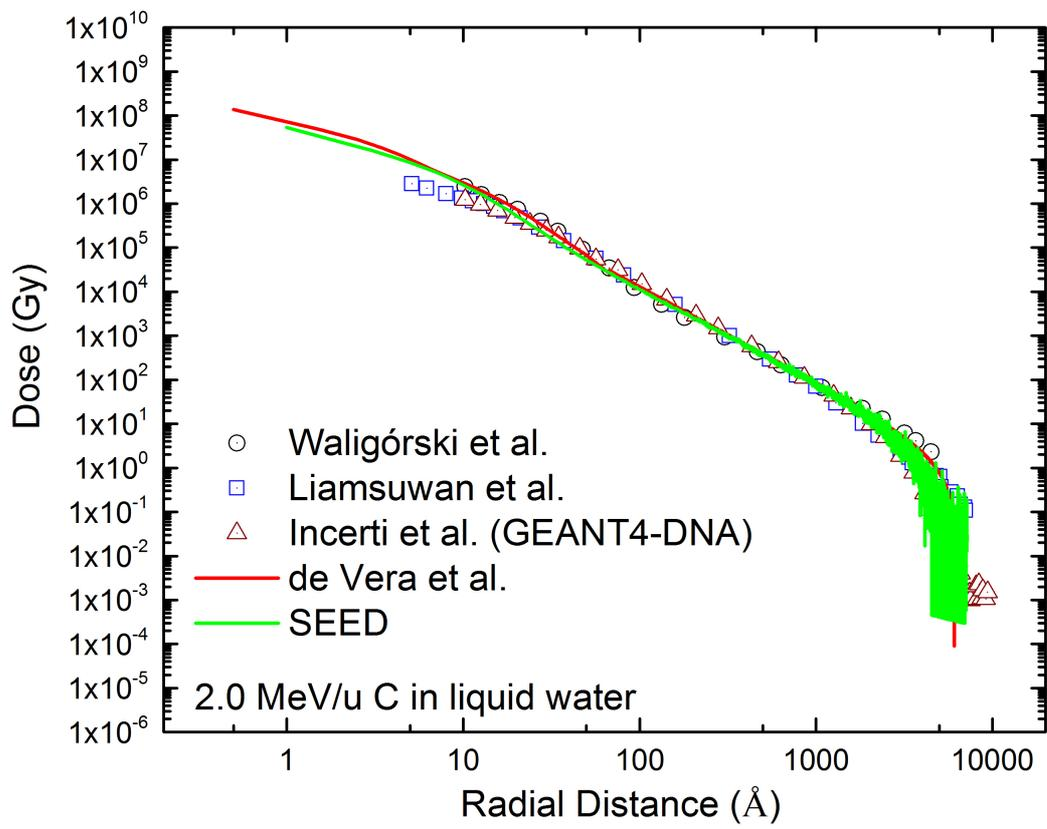
FIG. 1. SEED simulation of the radial dose around the track of a 2 MeV/u carbon beam incident on liquid water compared with the results of other authors [8-11].
