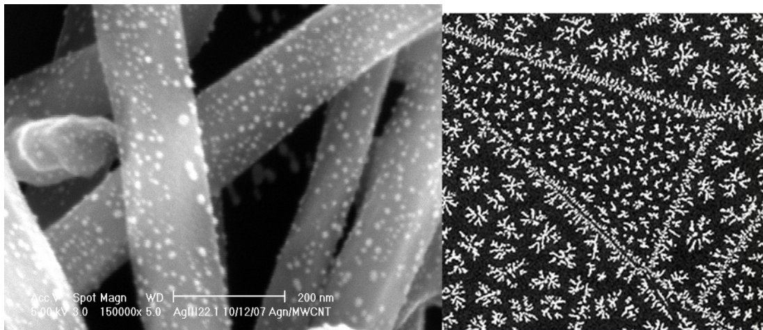
figure : SEM Images of clusters deposited on MWCNT (left) and HOPG (right) showing defect marking and grain boundaries determination as an example
