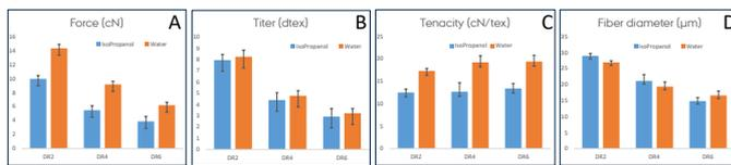
Figure 6: Technical testing of manufactured cellulosic fibre
