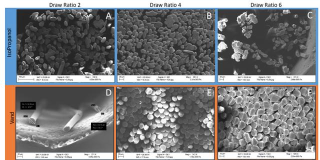
Figure 5: Scanning electron Microscopy of manufacture cellulosic fibre.
