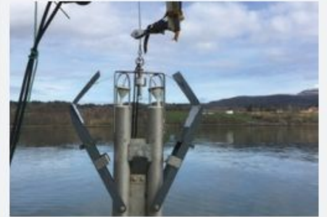
Sediment samples from Frænfjorden (left) where taken using a Gemini corer (right). Photo: E. Ramirez-Llodra (NIVA).
