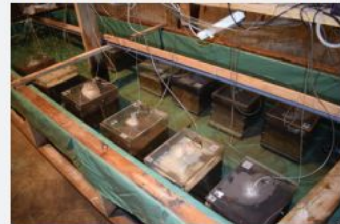
Mesocosm experiment where benthic fauna is exposed to mine tailings. Photo H.C. Trannum
