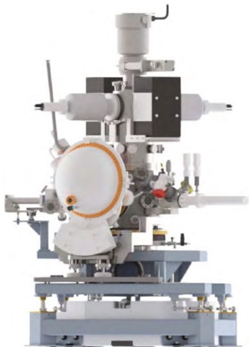
Figure 1: A model of the SGM4 spatially resolved ARPES endstation
