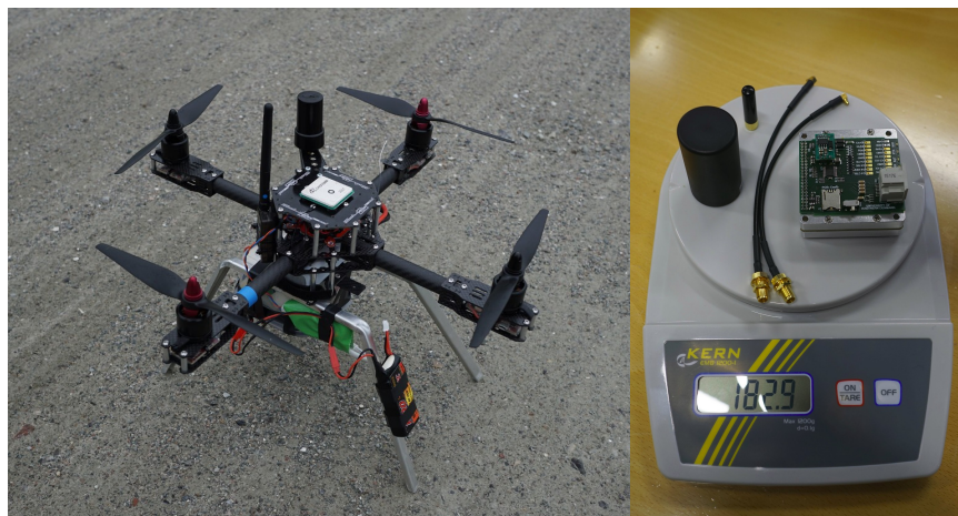
Figure 1: (a) The EduQuad drone used in this work. (b) Trimble BD920 RTK GNSS with the external interface board. The total weight including the GNSS antenna, a small stubby GSM antenna and antenna cables is 183 g.
