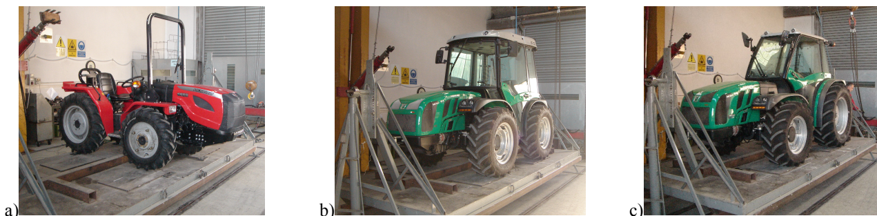
Figure 2. Tractor positions on the oscillating platform for longitudinal and transversal moments of inertia calculation. a) front foldable two post ROPS, b) square Cab ROPS, c) round Cab ROPS
