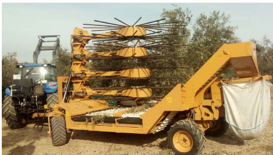
Figure 5. Harvester working around a traditional olive tree
