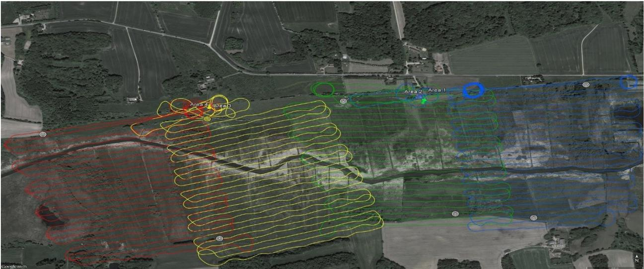
Figure 1: Example of the four flights covering area 1 to 4 equal to approximately 150 hectares.
