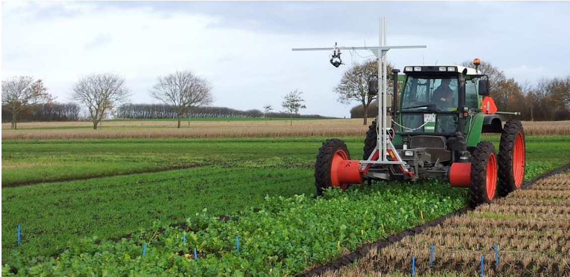
Figure 1. Photograph of experimental setup mounted on a tractor. The camera was mounted to one side, since the plant samples were taken from the side of the plot experiment. Each plot was visited twice in order to photograph both sides of the plot.
