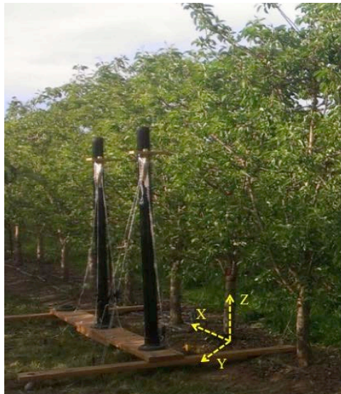
Figure 1. A wooden frame carried six digitizer ‘source’ modules, in order to cover the volume of large trees.
